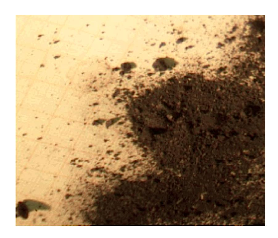
Above: Dust from a failed fuel rod, from US NRC NUREG 2121, Fuel Fragmentation, Relocation, and Dispersal During the Loss-of-Coolant Accident, 3/2012
