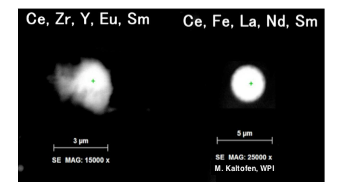
SEM analysis showed that the majority of the radioactively-hot particles detected were 10 um or less in size, meaning that they were potentially inhalable.
